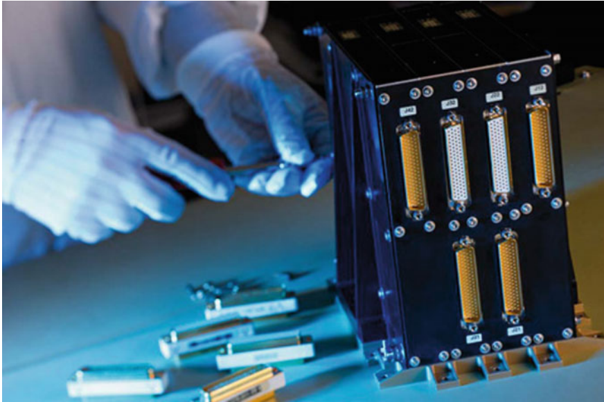
Fig. 4 OSCAR flight OBC during final integration (courtesy AIRBUS)
