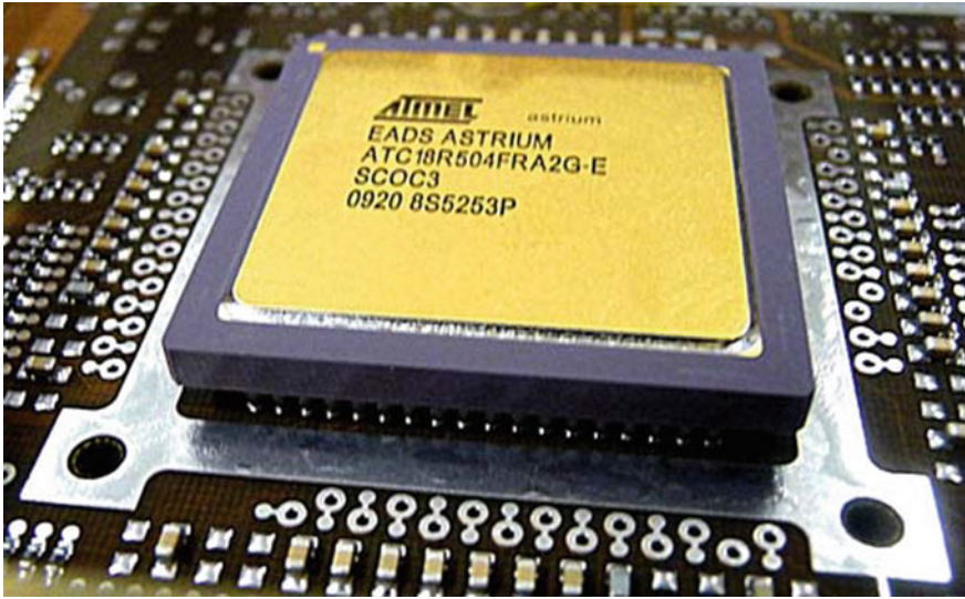
Fig. 5 SCOC3 ASIC (courtesy AIRBUS DEFENCE and SPACE)
